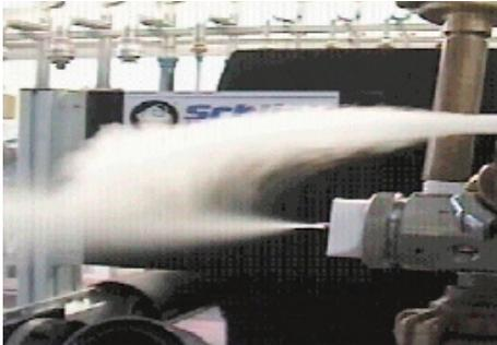
Image 2: Dust particles are kept away from the new air cap, instead of adhering to it
