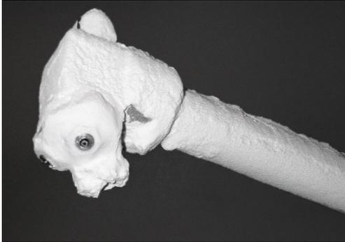
One of the old, blocked multi-head nozzles. It is no longer possible for fine droplets to pass through the heavily coated orifice areas; the thick film can also break off.
