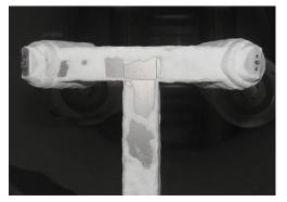
The new nozzle solution mod. 930/7-1 S68 after use. The orifices of both nozzles are clear and the spray is properly produced.
