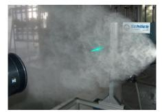
Spray from a flat jet two-substance nozzle
